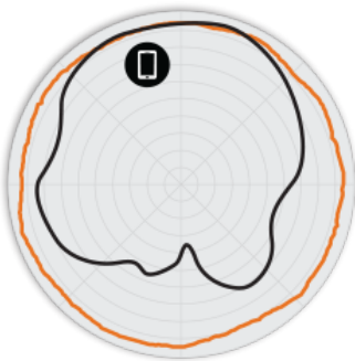
Figure 2. R600 2.4GHz Azimuth Antenna Patterns
