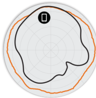
Figure 3. R600 5GHz Azimuth Antenna Patterns
